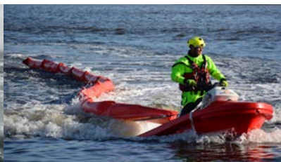
Pull oil booms or carry out other environmental protection operations.
